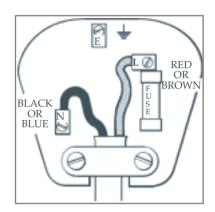
The wires in the mains lead are coloured in accordance with the following code: BLUE - NEUTRAL
